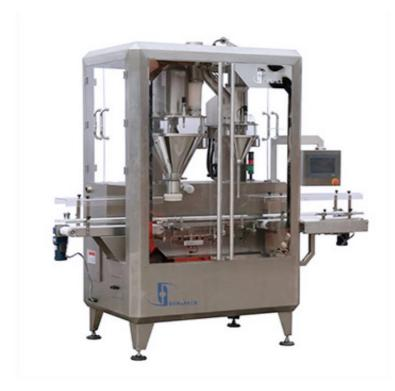
Automatic High Speed Powder Filling Machine Designed to fill high value powder like milk and protein powder into plastic bottle or metal cans. Line speed can be up to 30-40Pcs/min. Two stages filling integrated with inline checkweigher. Featured with high speed and good accuracy
