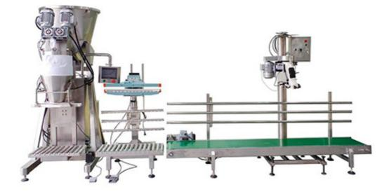
The Semi-automatic Open-mouth Bag Filling Machine also called semi-auto Auger Filler is OEM designed for Europe Agent. It can be applied to the quantitative measurement of a variety of powders or fine particles with big dosing 15-50 kg such as flour, coffee powder, milk powder, tapioca flour, seasoning powder, chemical powder and other materials.
