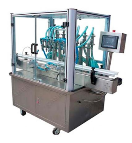
Automatic hand sanitizer filling line including hand sanitizer bottle filler, capper, induction sealer, etc. It can fill different shapes of bottles also we offer specially attachment gives you the options to bottles & shapes, including rounds, wide mouths, narrow mouth, cosmos, cylinders, oval, oblong and plastic jug. Plastic bottle materials include PET, LDPE, HDPE and PVC filling machine, capping, and labeling machine.
