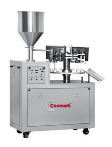
This machine is mainly used for quantitative filling and end-sealing of metal tubes as packaging container materials, and it is widely used in packaging in medicine, daily chemical, food, chemical and other industries.
