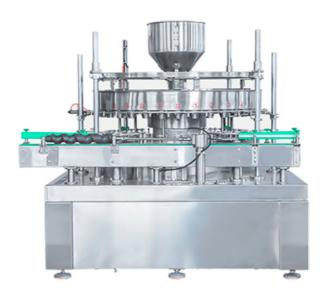
Based on digesting and absorbing domestic and international same equipment, the machine is specially designed for rationed filling of mixed materials. It is suitable for small volume filling. It adopts the telescopic rationed filling mode and its volume is precisely adjustable.
