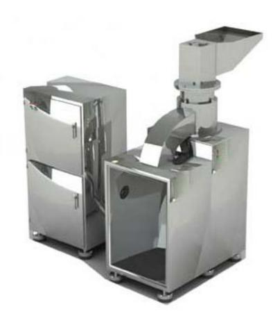
WCSJ Series Dust Collecting Coarse Crushing Set is applied as supporting equipment before fine crushing process in the field of pharmaceutical chemical and foodstuff etc., WCSJ Series Dust Collecting Coarse Crushing Set is a new generation coarse crushing equipment combining crushing and dust collection as a set of machine.
