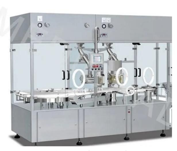
The servo motor is used to control the number of driving circles of the screw conveying powder, so as to accurately control the raw material powder to be packed into the silverbottle according to the required capacity and cover the rubber stopper tightly.
