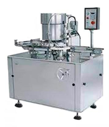
KGL-1 is the first generation of roller capping machine which our company has developed by referring the similar product in domestic market. After several innovation, it is deeply welcomed by pharmaceutical factory users. It is suitable for the capping of round glass bottle and plastic bottle. It is used in pharmaceutical industry, light industry and chemical industry.
