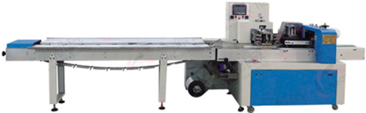
Using original single servo or double servo motor control, compared with other domestic and foreign similar inverter motor or inverter control products, more intelligent, higher packaging precision, wider adjustable range, more accurate control, lower scrap rate and better stability. Due to the full open box structure, the transmission structure is clear at a glance, and the maintenance is more convenient;
