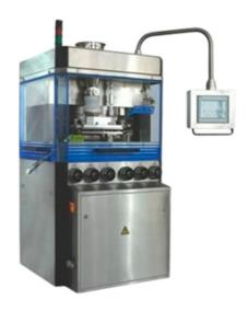
ZP4100 Rotary Tablet Press is a serial product widely used in pharmaceutical, food, chemical and electronic industry to produce all kinds of round tablets, irregular and double side engraved tablets.
