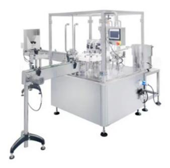
This machine uses rollers to sort and load bottles, a disc to position the peristaltic pump for filling, a cap sorting disc to vibrate the lower cap, and a capping head to cap. The structure of this machine is compact, reasonable, easy to maintain, and can be easily linked with other equipment to form a line.
