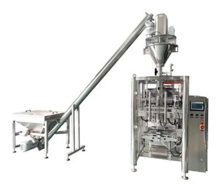
This powder packaging machine completes the whole packaging procedure of measuring, loading materials, bagging, date printing, charging (exhausting) and products transporting automatically as well as counting. can be used in powder and granular material. like milk powder, Albumen powder, solid drink, white sugar, dextrose, coffee powder, nutrition powder, enriched food and so on.
