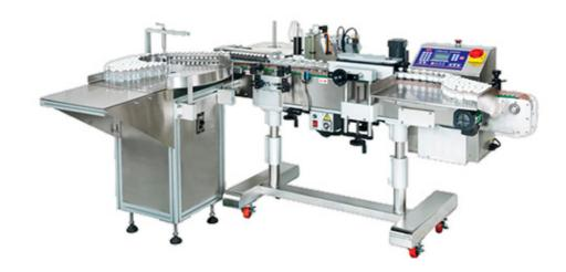
The labeling equipment CJL-2000 series is suitable for self-adhesive labels for round bottle wrap around procedure.
