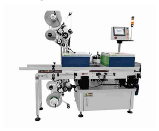
Loading→Separation→Deflection→Upper and lower labeling→Side labeling→Pressing→Online inspection and removal→Finished product.
