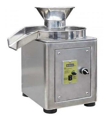
ZLB80 Rotating Granulator is a mini wet rotating granulator for research and development. The performance of the machine, such as formability and disintegrating performance, can be easily discovered only by about 30 gr. powder lot. The machine can produce cylindrical granules with diameters of 0.8, 1, 1.2 and 1.5mm, and the produced granules are neat and beautiful.
