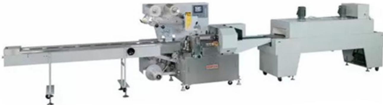
The shrink film horizontal packaging machine uses heat shrink film to wrap products, which shrinks tightly around the item when heated, achieving a sealed and visually appealing packaging effect. This machine is widely used in industries such as food, beverages, daily necessities, medical devices, and industrial products.
