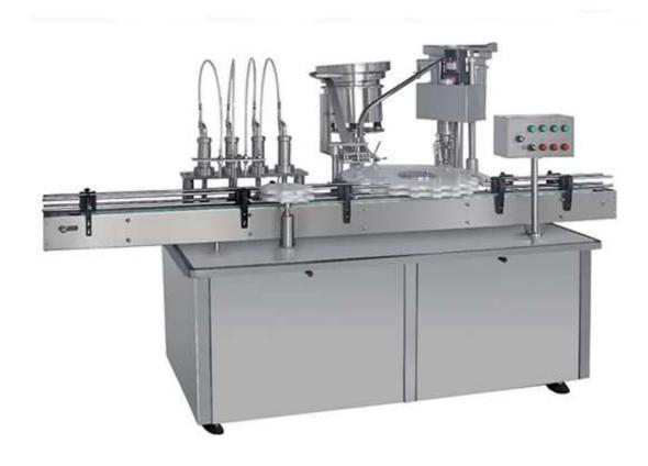
The machine is applied for filling and capping glass bottle, plastic bottle from 30ml to 500ml.
