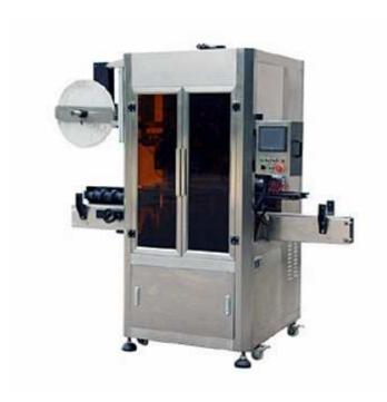
BSL-100M type is a kind of low-speed machine, but it adopts equivalent PLC, positioning module, servo motor and frequency converter. Besides, its touch screen is featured with a humanized operation. It adopts PLC programmable controller, imported servo motor, servo driver, frequency converter and transducer; besides, it adopts the positioning module to ensure the casting label precise, rapid and stable.
