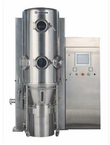
Drying: The high drying efficiency is because the powder or granules are fluidized in the drying chamber and the container is using a turbo blower, the hot air passed through the powder or granules from bottom to the top of drying chamber to remove the humidity.
