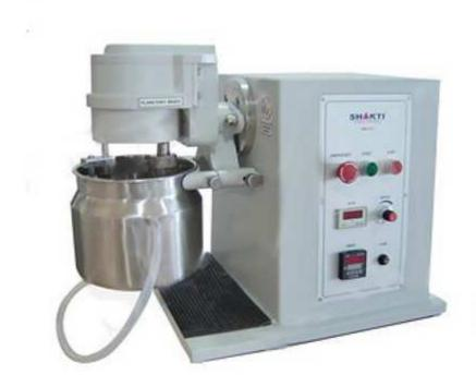
This mixer is designed to be used as a mixing for pastes, ointments & creams in water-jacketed kettle. It can also be used for wet powders. This mixer is provided with a mixing paddle and Teflon scrapper, which is shaped in such manner so that there is minimum clearance with the mixing kettle. The kettle is also easily removable.
