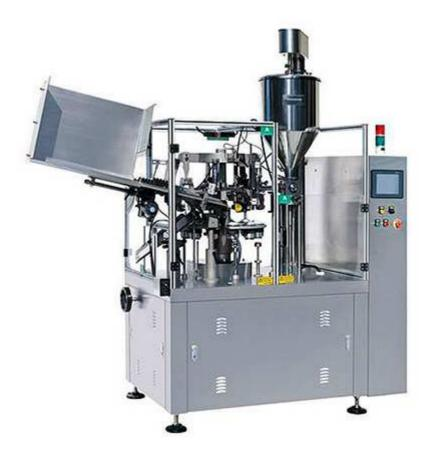
VF-80Z Metal Tube Filling and Sealing Machine can be used in the industries of pharmaceutics, foodstuffs, cosmetics, daily chemicals for smoothly and accurately filling all kinds of pasty and viscous fluid and the materials alike, into soft metal tubes and then carrying out tube end folding, sealing and lot number printing.
