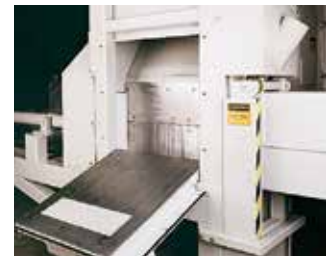
Densification chamber (door open)
