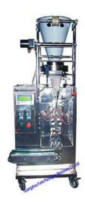
It is wildly used in medicine, foodstuff, the chemical industry of grain, pills, powder, etc. All the works of bag-making, date printing ration filling, sealing-cutting. It is made up of stainless steel and up to International Health standard. The machine is reliable and operates easily, few stoppages. It has a good reputation in home and abroad.
