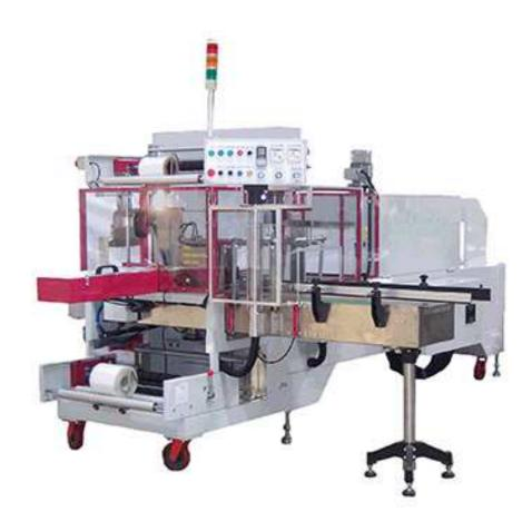
SA-116 sleeve type sealing machine (including shrink tunnel) is suitable for group packing bottles, such as water, beverage of canned food. Available with transparent PE shrink film (each Top and Bottom film cradle) OR printed PE film (only Top film cradle) Easily change the package matrix among modules. Its speed could up to 14 packs per minute based on 330ml can by package matrix of 3x2.
