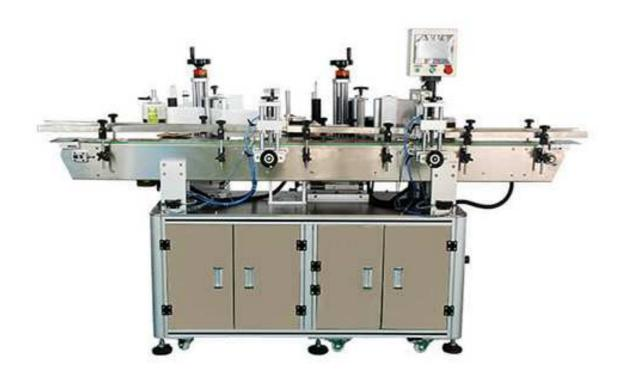
HL-T-408 this labeling machine is specially designed with unique specificity. It is dedicated to round bottle wrap around labeling or positioning labeling. After the user is familiar with the equipment operation, they can do labeling for other round bottles, such as food can, cosmetic round bottle, medicine bottles etc.
