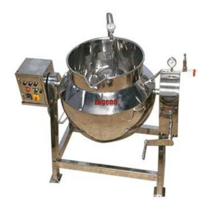
Starch paste kettle designed for application in pharmaceutical processing units. Used For Preparation Of Starch Paste. Conical Shape Ensures that the Heating Of the Starch Paste Is Uniform And Gets More Surface Area. The Tilting Type Arrangement Ensures Ease In Unloading The Paste Into Any Container Or Vessel.
