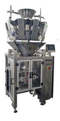
The machine can complete various functions including quantitative weighing, automatic feeding, film forming and bag making, automatic sealing, automatic punching, automatic printing date cutting and counting.
