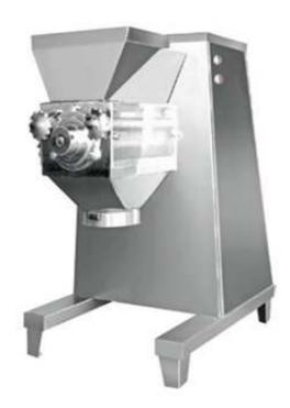
This machine is used mainly in such trades as pharmacy, chemical industry, food, pottery and plastics extensively, making moist powder material particle. Make cylinder swing reciprocally, extruding material from screen mesh for granulation.
