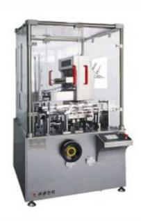
This machine is suitable for cardboard case packaging of blister packing for capsule and tablets. It consists of direction folding (1-4 folds) and feeding equipment, cardboard case forming and feeding, batch number printing, sealing of case tongues at both ends ect. The whole encasing process is finished automatically. It can be added hot-glue machine.
