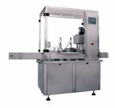
Bottle feeding, filling and plug putting are on dual rails; linear bottle feeding; liquid level filled can be tracked and controlled by stainless steel valve to ensure there is no adherent liquid and dropping liquid; detect with optical fiber; plug putting by cylinder; stop putting inner plug with no bottles there; percent of pass of putting plug is high.
