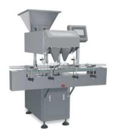
The bottle blocking of bottle feeding mechanism's track stand bottle filling position and wait fill from the last equipment. Drugs through the corrugated plate vibration, orderly into drug storehouse. And the drug storehouse is equipped with photoelectric sensors, the drug fall into the drug storehouse were putted into bottle by photoelectric sensor quantitative count.
