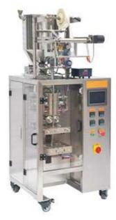
This model machine for sale vertical form fill seal stick pack machine is suitable for packaging tea, coffee, Chinese medicine pieces, and other similar products. It can automatically sachet forming, measuring, filling, sealing and cutting into sachet.
