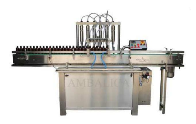
The incoming dry bottles (sterilized and silicones) are fed through the in-feed turn table and suitably guided on the moving SS/Plastic slat conveyor belt at the required speed of the correct placement below filling unit. Bottles in a raw are held by pneumatic stoppers at a time below the filling nozzles. During the stationary position, the set fill volume is delivered into bottles.
