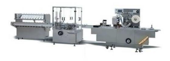
This machine is suitable for scatch, punch, soft al/al strips, wound pester, ointment plaster, facial mask, coffee bags, condom bags into carton automatically. On line product feeding and detecting, carton opening and forming, products and leaflet push into carton, printing batch number, sealing carton with tuck-in or hot melt glue device. Automatically reject lacking of leaflet or product and finished product out.
