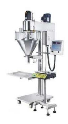
This machine is suitable for packaging fluidity Powdery product like milk powder, albumen powder, solid drink, white sugar, dextrose, coffee powder, rice powder, fodder, pharmaceuticals, agriculture pesticide, granular additive, dyestuff etc in bag, can, bottle package. Stainless steel design, in line with GMP standard, It can do measuring and filling work.
