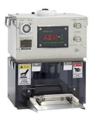
ABM-I blister packing machine is our newly developed pneumatic blister sealing machine. On the basis of the previous manual blister sealing machine, the machine enlarges the mold size, has a precious sealing timer, and adopts cylinder for sealing, which provide sufficient for sealing and makes sealing easier. Hence, it improves the product quality and production efficiency.
