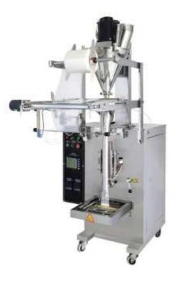
Automatically measuring volume, making bags, filling, sealing, cutting, printing the lot number and cutting easy tearing notches, making chain sachet, finished product conveying.
