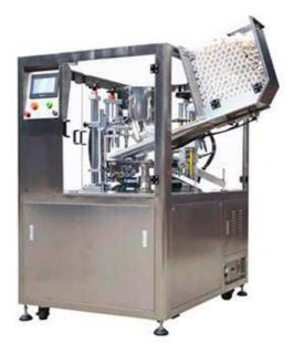
This filling and sealing machine is widely used in pharmaceutical, cosmetic, food and chemical industries etc., it is applicable in various aluminum plastic compound soft tube, plastic soft tube which fill pack all kind of Such as ointment, adhesives, AB glue, Neoprene, epoxy glue, skin cream, hair cream, boots oil, toothpaste and else liquid, lotions and cream etc.
