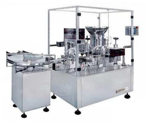
This vial bottle filling capping machine contains processing of feeding, filling, plugging and capping. The machine meets GMP requirement with high efficiency and anti-leaking function. Easy operation with PLC controlled and adjustable parameters in touch screen. Each machine can be used stand-alone, also can be used for filling line. It is widely used in pharmaceutical, biology, health care industires.
