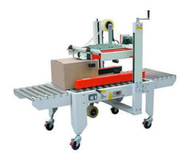
FXJ-8060B heavy-duty case sealer is based on the standard model, the frame is enlarged, and the driving belt is installed more, so that the equipment can pack heavy and large goods. Generally, the items with weight more than 25kg need to be purchased this heavy duty sealing machine
