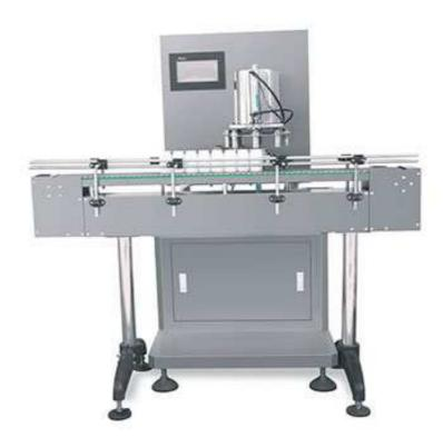
Automatic cotton inserting machine suitable for all kinds of grade and weight cotton strips. The sliver is pulled out by the pressure wheel controlled by the motor, and then the cylinder movement, the cotton is packed into the bottles with the U-type.
