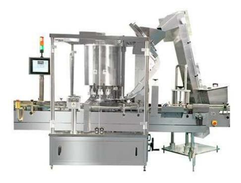
Equipped with three pairs of friction wheels, self-adjust tightness, helpful the caps surface. Wide applicability, it is simple and convenient if change bottles and caps, just, adjust some components. Equipped with human-computer interface and PLC control system, Ensure more stable operation and easier handling. Self-diagnose errors and stop working to make alarm at errors and missing bottles caps. The bottle with twisted cap, anti-cap and without aluminum foil will be removed.
