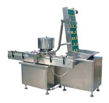
This plastic and glass bottle screw capper employs elevator to feed bottles and its capping head can automatically seize and screw caps. In this way, it enjoys high automation degree.
