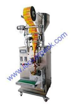
This machine is suitable for pharmaceutical, cosmetic, food and chemical industries particles pouch packaging. Such as Radix, cold particles, desiccant, coffee, detergent and other granular materials.
