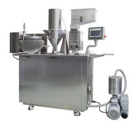
Semi-Automatic Capsule Filling Machine can fill up to tens of thousands capsule per minutes. It only requires one person to operate machine which is simple to start with and has high filling efficiency. With the replacement of the mold, you can start safe production of 00,0,1,2,3,4,5 size capsules. What's more, we could provide an ultra-quiet version for our customer who has special need for sounds.
