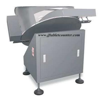
Our company is specialized in pharmaceutical and food machinery in China. This machine is equipment that can automatic packing bottles automatic transport bottles. This type is suitable for plastic bottle sorting, can make different size different type plastic round bottles.
