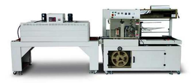
The machine is mainly aimed at mass heat shrinkage packaging of cosmetics, printing products, pharmaceuticals, electrical appliances, food, beverage, hardware and plastics, and is used in conjunction with the jet heat shrinkage packaging machine to achieve complete and good shrinkage effect of packaging items.
