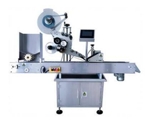
For standing firm circular cylindrical objects, semicircular labeling, the use of horizontal transmission, horizontal labeling way to increase stability, improve the labeling efficiency.
