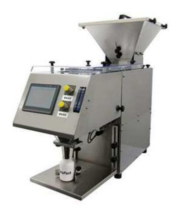
TM-100 counter is designed to feed and count any size, shape or quantity of tablet and capsule without change parts.
