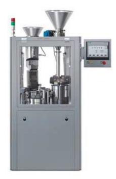
NJP-800C Automatic Capsule Filling Machine adopts butterfly valve-type powder feeding, and is very suitable for drug powder with poor liquidity, including Chinese herbal medicine and Chinese patent drug, due to that its vibration unit equipped will force the powder to run down, which has solved problem of failing to feed in powder that often happens in the traditional screw feeding device because of the poor liquidity of powder.
